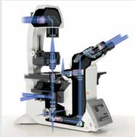
Opto-mechanical documentation of the Infinity Port
