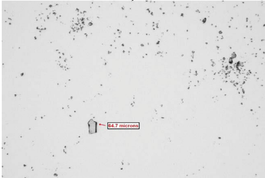
Figure 1. Field of view showing the longest particle found in the analysis.
