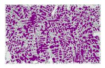
MLDS is an approach based on an image analysis routine which automatically detects dendrites, superimposes a set of concentric circles and exports measurements of overlapped features.
