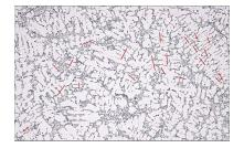
The manual SDAS method using a Clemex system involves capturing images from a sample and annotating a number of secondary dendrite arms with direct measurement tools.
