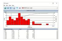
The length distribution of these manual measurements is updated instantaneously in the results panel of the software and can be exported for further processing using a Linear Intercept Method macro to obtain DAS.
