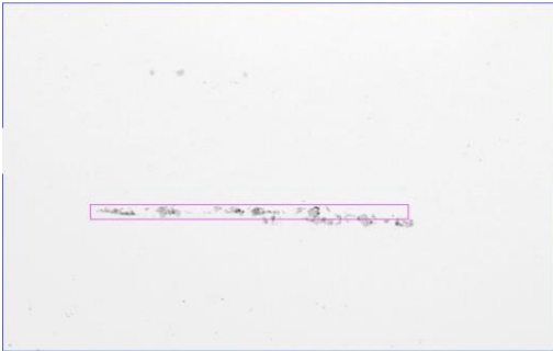
Figure 2: The inclusion was reconnected and classified as an alumina stringer (OA).
