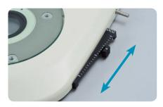
The OCC illuminator can be controlled using a slide lever. Thanks to scales on the slide lever, the user can save and reproduce desired illumination levels. In addition, an OCC plate can be inserted into the illumination unit from the front and rear sides, so images with different shadow direction can be observed.
