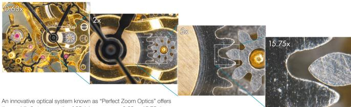
the world's first zoom ratio of 25:1 (zoom range: 0.63x - 15.75x\*; \*as of May 2013). The SMZ25 can seamlessly capture the entire dish while simultaneously delivering microscopic details.
